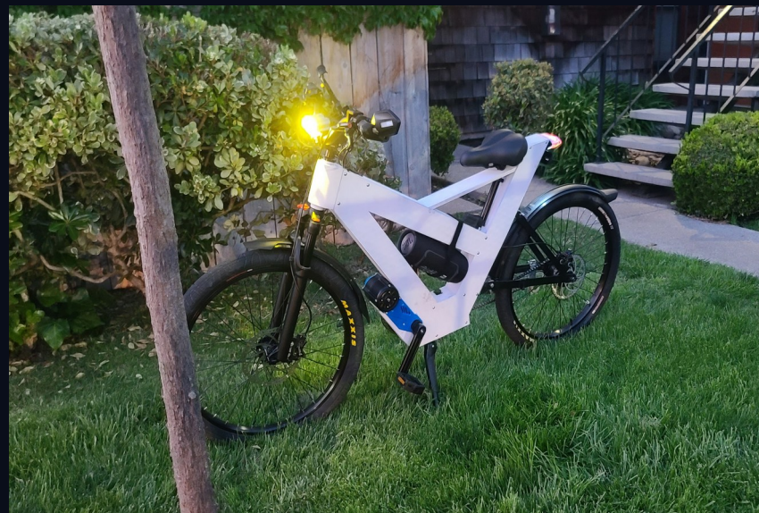
Prototype 2 — White | 3D printed chevron frame | Running lights | Operational
