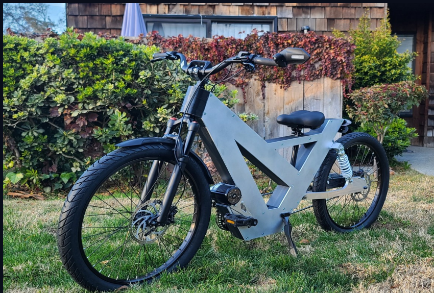
Prototype 1 — Silver | 3D printed chevron frame | Aluminum side plate | Operational
